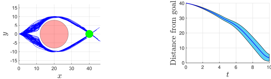
(a) Paths followed with path integral controller (b) Mean distance from goal \pm standard deviation
